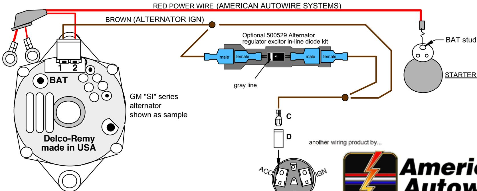
**INSTALLATION OF POWER WIRE - ALL ALTERNATORS**
