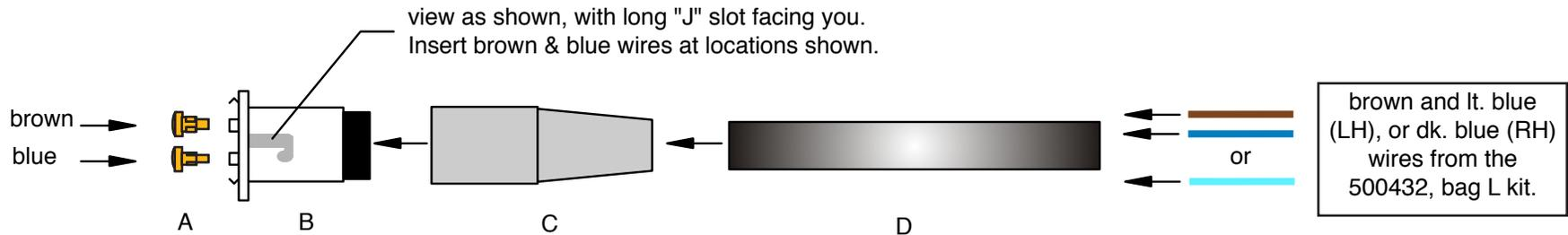
1. It will be necessary to do an in-line splice or other type of connection on the brown wire, as it must be used for both the LH and RH parking lamp assemblies.
