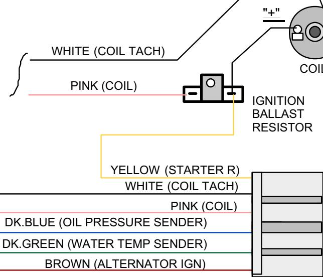
THIS 6 POSITION FEMALE CONNECTOR IS PLUGGED INTO THE MATING 6 POSITION MALE CONNECTOR LOCATED IN THE FUSE PANEL ASSEMBLY!!!
