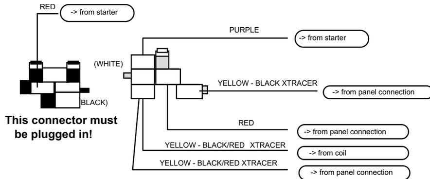
Connecting to a GM column mount switch connector using supplied terminals. American Autowire has GM connectors available.
