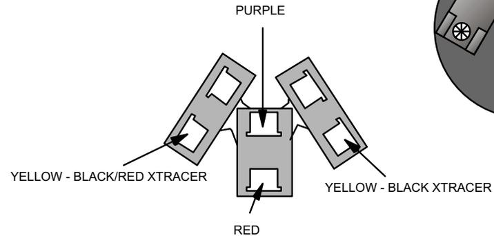
1. Plug all wires into the supplied BLACK connector as shown above. **IMPORTANT** - note orientation of wires before plugging into connector!
