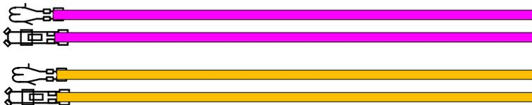
**PURPLE / YELLOW WIRES:** If you are using an electric speedometer, it will be necessary to use these wires for the speedometer sensor. Each wire has a mating terminal to the other (same color) wire. Plug the female into an unused cavity in connector A. Plug the mating male into the mating cavity on the dash harness connector. Route the other ends to your speed sensor and speedometer, and connect per the manufacturer's instructions.
