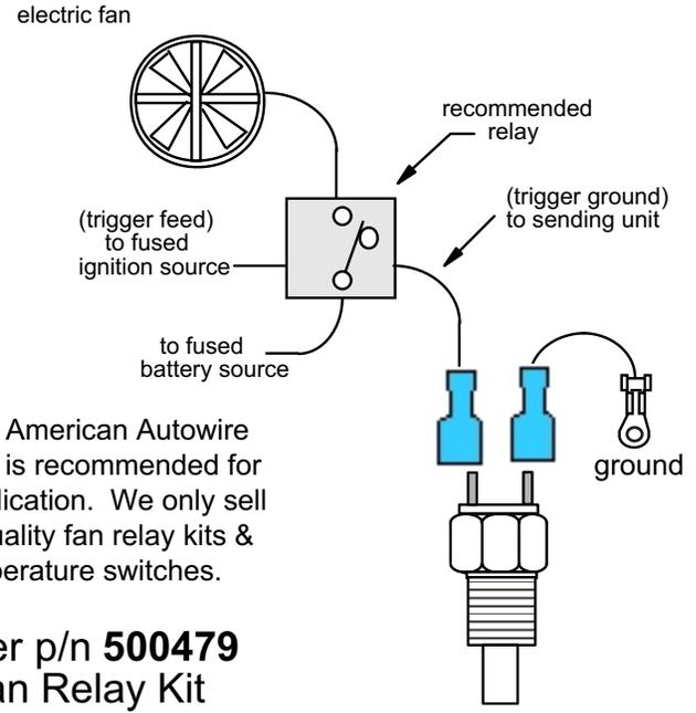
Apply anti-seize compound to the female threads in cylinder head or manifold before installing your new sensor. DO NOT overtighten! Sensor has tapered standard pipe thread (NPT) that self seals by design. DO NOT use pipe sealants or teflon tape. Use only with coolant containing corrosion inhibitors or antifreeze. Damage to sensor from overtightening or excessive corrosion voids warranty.
