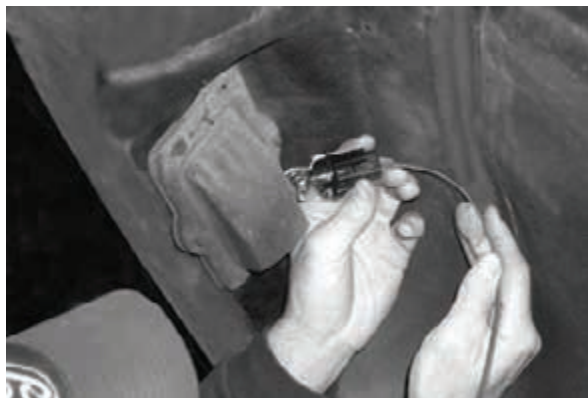
Plug the lamp socket with the lt blue / brown into the driver's side lamp assembly, and the bk blue / brown into the passenger side.
