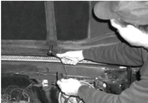
Remove driver side hood support.
