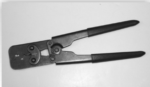
Double crimp tool. Used for larger gauge terminals and double wire crimps. p/n 500523 .....$89.95
