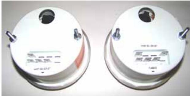
AutoMeter 3 3/8 inch Series I tachometers (left) and speedometers (right) are lit with a twist in light socket. The lamp power connection is made within the 8 cavity gauge connector on the LAMP terminal.
