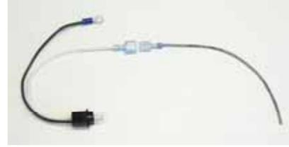
Light sockets for Series I gauges are provided separately. This kit includes separate male and female disconnects and ring terminals that are used to connect the light sockets to the harness assembly. This picture shows the correct way to terminate the light sockets with the enclosed terminals.
