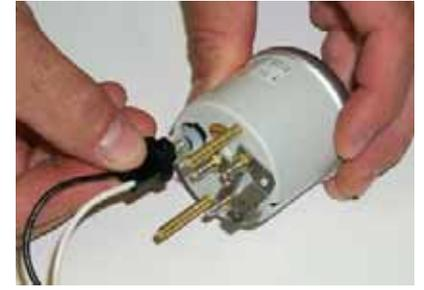
**STEP 4:** Install appropriate lamp socket pigtails into the speedometer & tachometer.
