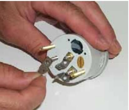
STEP 2: Install the blade terminals to the back of each of the 4 small gauges. Secure with lockwasher and nut. There are specific left, center, and right hand terminals. Install as shown in photo.
