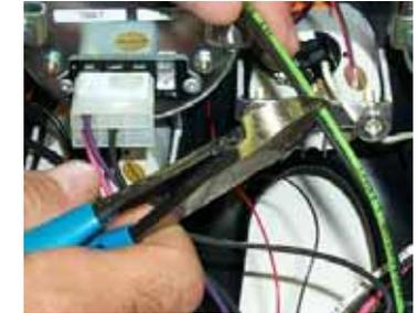
STEP 12: Install butt connectors, as shown, matching the wire functions noted above with the proper LED. Trim the wires from the harness to the desired length before crimping.
