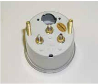
STEP 1: There are 4 small gauges. This is a photo of the bare gauge. Remove the 3 nuts and lock washers.
