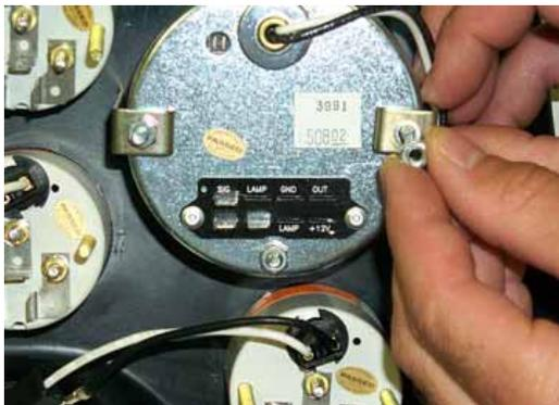
STEP 6: Install mounting clips on tachometer & speedometer.
