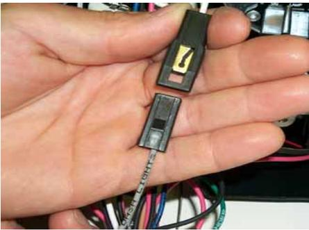
STEP 11: Plug each lamp power wire (white) into the mating connectors on each grey wire (DASH LIGHTS) on the new harness. As shown.
