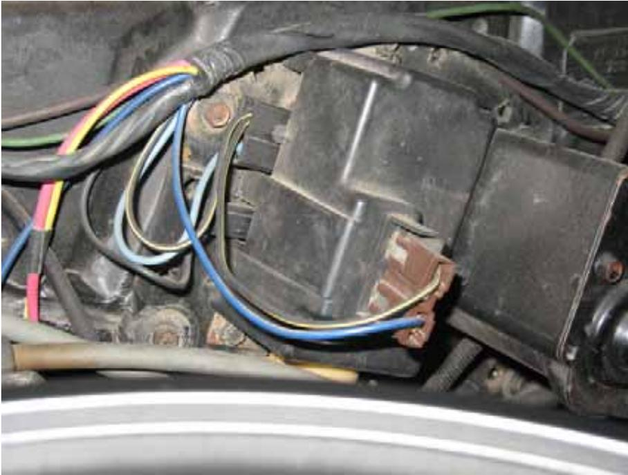
The photo above depicts the typical stock 1967-1969 Camaro (all), 1968-1972 Nova (all), 1967-1968 Firebird (all), and 1970-73 Camaro “without depressed park” wiper motor and washer pump connections. Where you see the black wire with the yellow strip in the photo, that would be equivalent to the AAW white “wiper feed” power wire.
