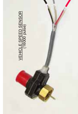
Typical 3 wire Autometer 5291 VSS connection
