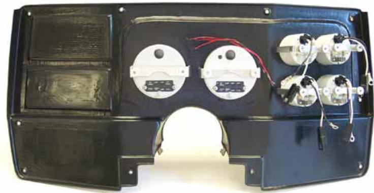
Complete gauge cluster assembly ready for wiring.
