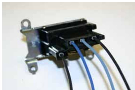
The above picture shows the orientation for 72 Nova wiper hook-up only. All other applications can only be plugged in one way.
