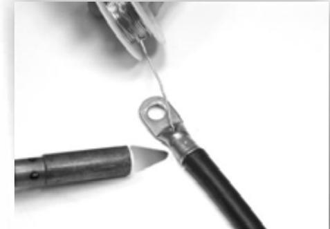
**STEP 6:** Remove the terminal from the vise and heat the crimp area of the terminal with a proper torch. Apply rosin core solder through the solder hole, as shown.
