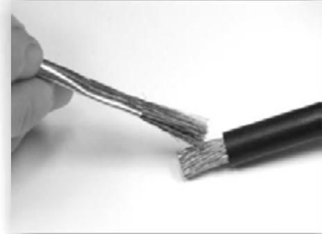
**STEP 3:** Strip the cable to 5/8", and apply rosin solder flux. A protective sleeve (shrink tube) should be slid onto the cable at this point if you are using one.
