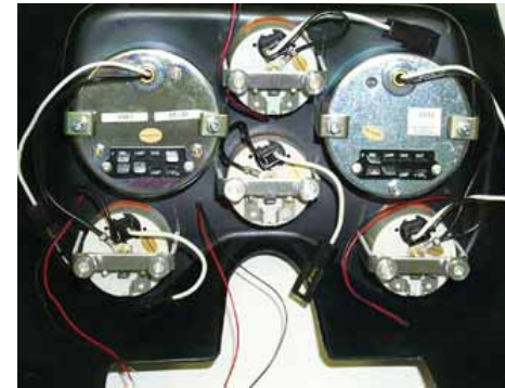
Complete gauge cluster assembly for 1976-78 Camaro ready for wiring.
