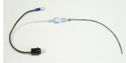
Light sockets for Series I gauges are provided separately. This kit includes separate male and female disconnects and ring terminals that are used to connect the light sockets to the harness assembly. This picture shows the correct way to terminate the light sockets with the enclosed terminals.
