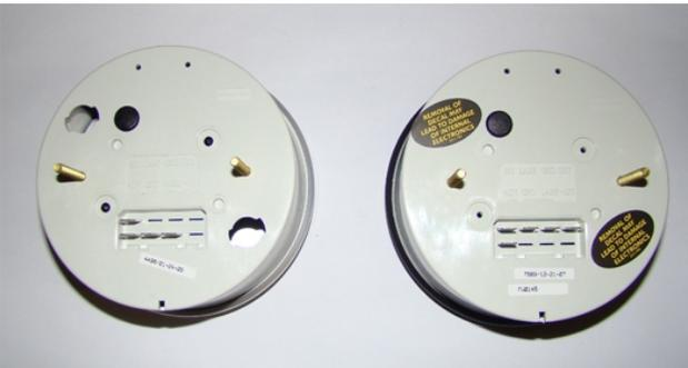
AutoMeter 5 inch Series I and Series II tachometers (left) and speedometers (right) have a LAMP terminal in the 8 cavity gauge connector. Series II gauges (on the right) require the light power lead to be on this terminal. Series I gauges (on the left) use separate light sockets and the LAMP terminal is not functional. Refer to the enclosed light socket connection photo to connect these sockets.
