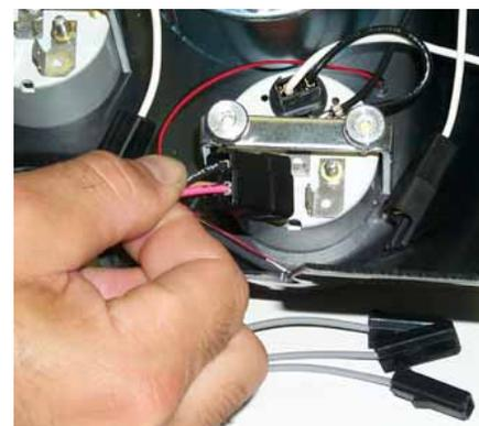
**STEP 5:** Plug in gauge connections using supplied connectors. Plug in connectors in the order shown below. A typical plug-in is shown in the picture.
