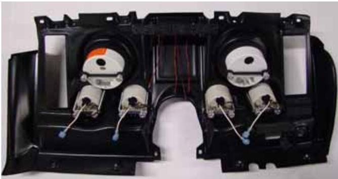
**STEP 2:** Install appropriate lamp socket pigtails into the gauges. Follow specific instructions for the tachometer and speedometer as there are several different lighting configurations.
