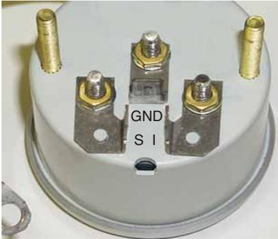
**STEP 1:** Install the blade terminals to the back of each of the 4 small gauges. Secure with lock washer and nut. There are specific left, center, and right hand terminals. Install as shown in photo.
