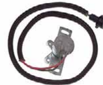
p/n 01993420 Muncie 4 speed back up lamp switch.
