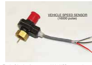
Typical 3 wire Autometer 5291 VSS connection
