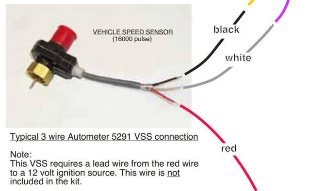
Typical 3 wire Autometer 5291 VSS connection
