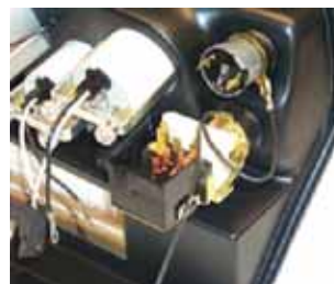
1968 Nova headlight and wiper switch grounding.
