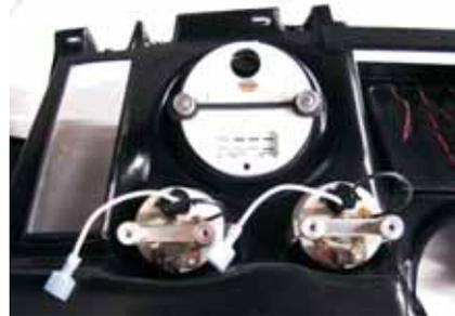
NOTE 2: This picture shows connection of lighting as would appear on Series II gauges. A separate blade terminal for power and ground exists for the internal lighting. The speedometer and tachometer have a specific lamp terminal within the 8 cavity plug.
