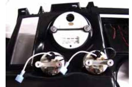
**NOTE 2:** This picture shows connection of lighting as would appear on Series II gauges. A separate blade terminal for power and ground exists for the internal lighting. The speedometer and tachometer have a specific lamp terminal within the 8 cavity plug.
