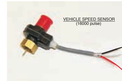
Typical 3 wire Autometer 5291 VSS connection
