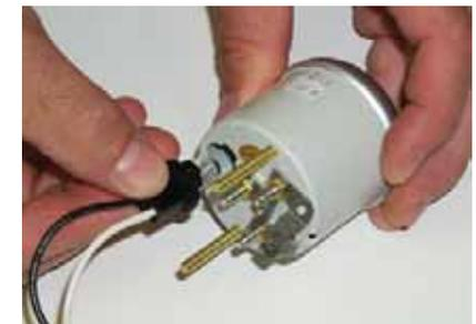
STEP 3: Insert the gauges into the housing in the locations shown.
