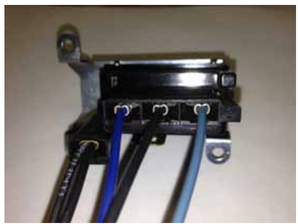
The above picture shows the orientation for 72 Chevelle wiper hook-up only. All other applications can only be plugged in one way.
