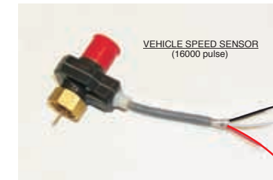
Typical 3 wire Autometer 5291 VSS connection
