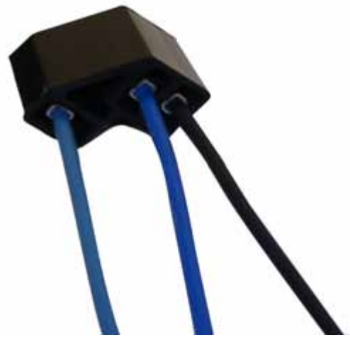
1968 wiper switch connection with depressed park
