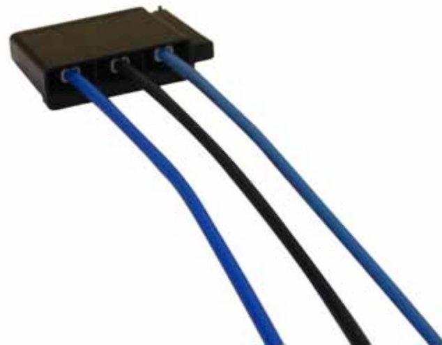
1969 wiper switch connection
