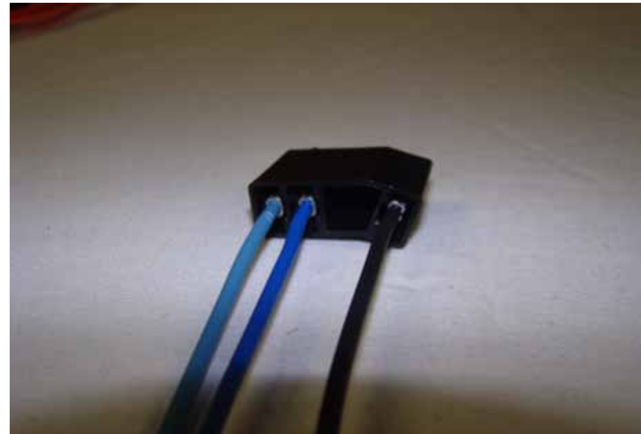
1968 wiper switch connection without depressed park
