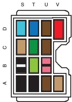
Temp. Gauge (engine connector location C-T)
