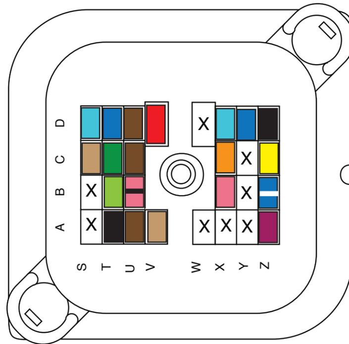
1968 - 1969 FUSE BLOCK BULKHEAD CONNECTOR
