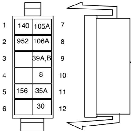
PLUG CONSOLE HARNESS CA97581 INTO THIS NEW CONSOLE GAUGE HARNESS EXTENSION CONNECTOR
