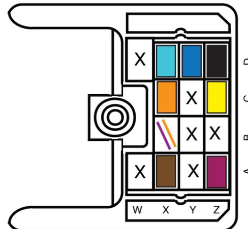
1968 - 1969 FUSE BLOCK BULKHEAD CONNECTOR
