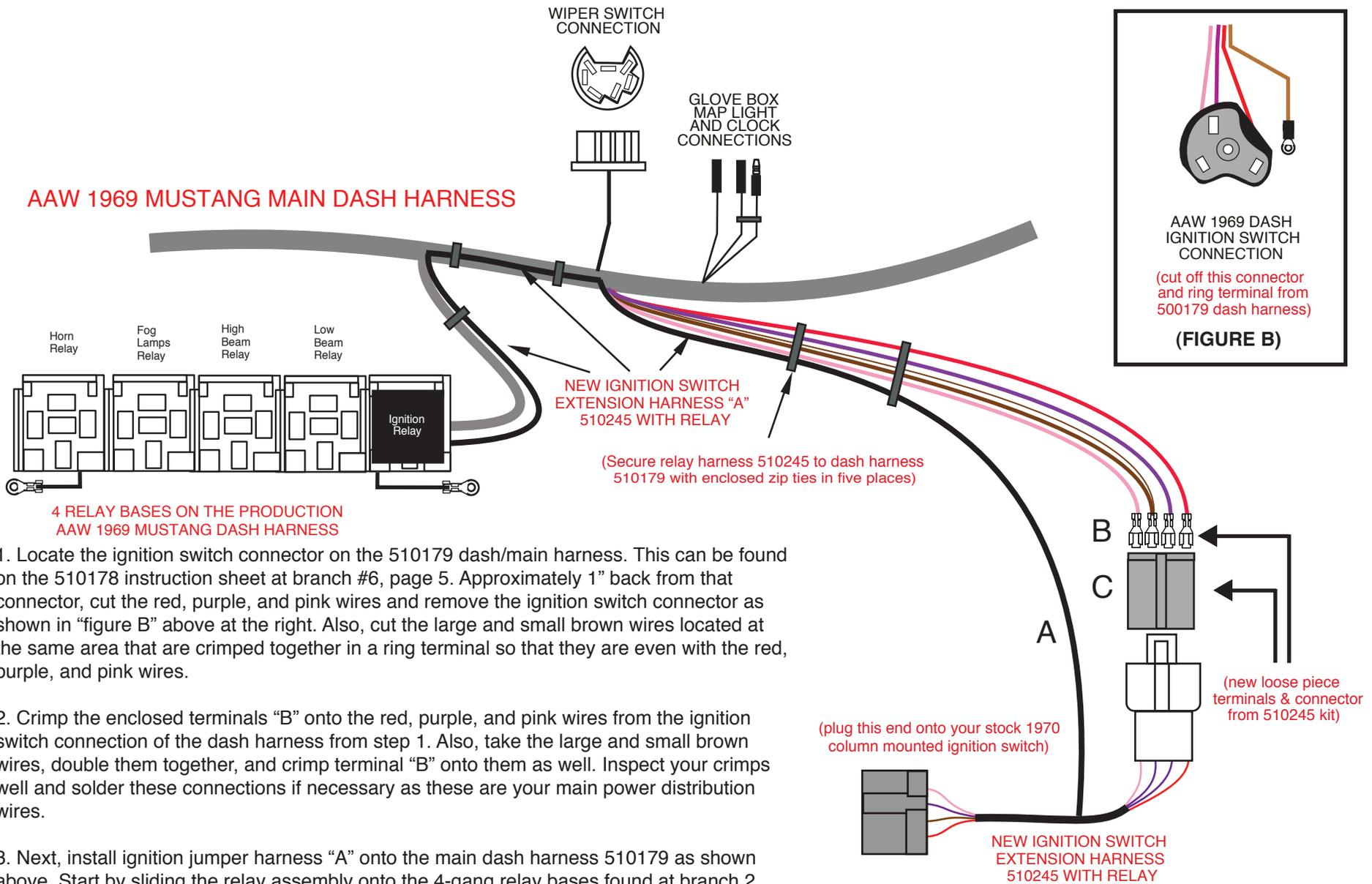
1. Locate the ignition switch connector on the 510179 dash/main harness. This can be found on the 510178 instruction sheet at branch #6, page 5. Approximately 1" back from that connector, cut the red, purple, and pink wires and remove the ignition switch connector as shown in "figure B" above at the right. Also, cut the large and small brown wires located at the same area that are crimped together in a ring terminal so that they are even with the red, purple, and pink wires.
