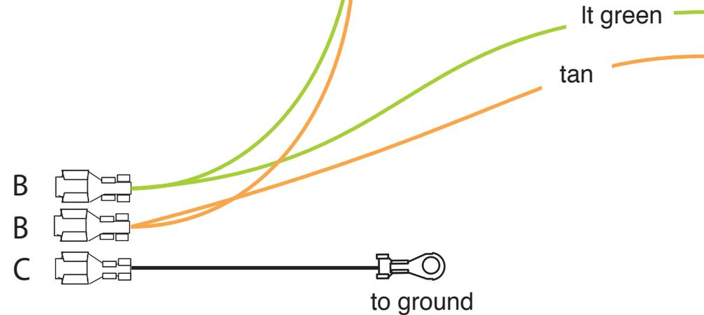
The 1970 Mustang utilized a single headlamp system as opposed to the dual headlamp system used on the 1969 Mustangs. On this sheet, you will find instructions that depict how to connect your headlamps. The function of each of the wires (lt. green, tan, and black) remains the same as on the main instruction sheet 510178, page 2, branch 2. AAW recommends that you use both this sheet and the 510178 sheet for installation of your headlamps.
