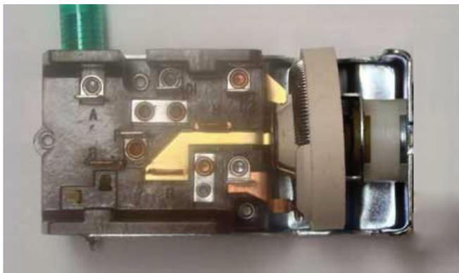
1. Install the new switch into your dash using the original bezel and nut. It will be necessary too cut the shaft for a nice custom installation.
