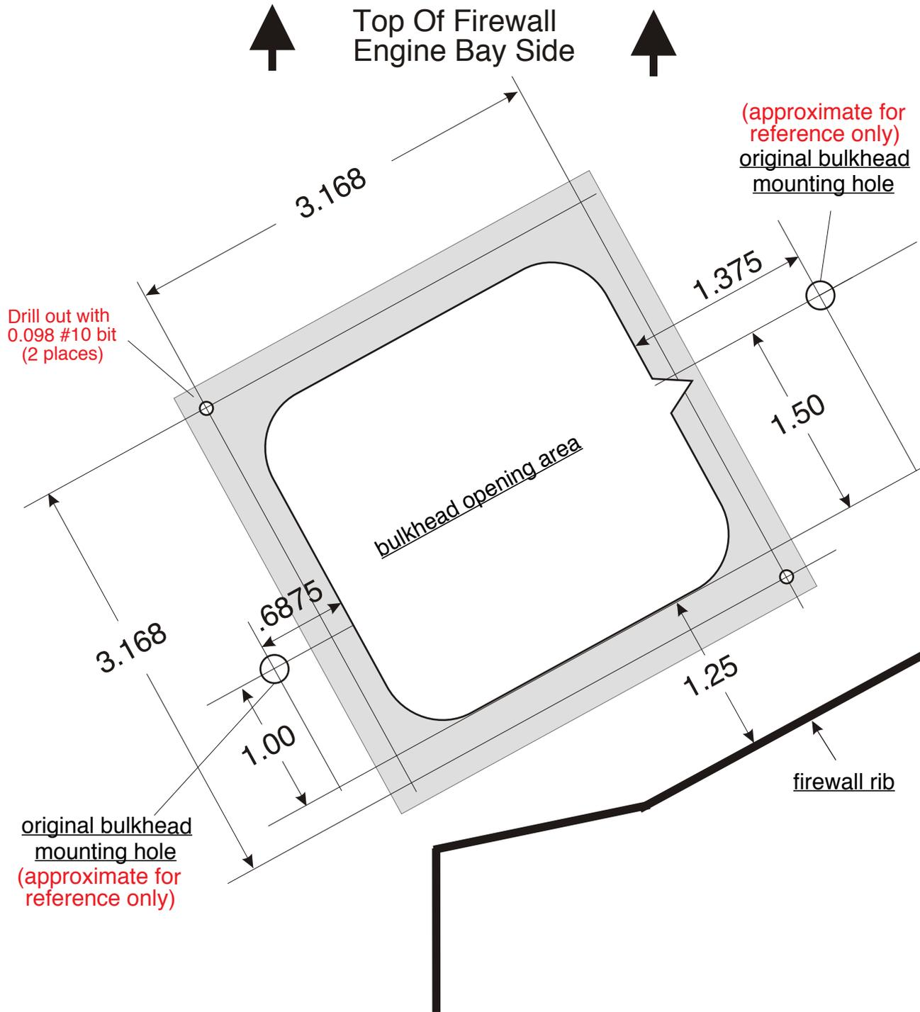
The only firewall modification needed with this new kit is to drill 2 new .098 mounting holes. The stock opening in the firewall is already the proper size for the new bulkhead assembly to fit through. This template can be affixed directly to the firewall or it can be applied to a stiff piece of cardboard or thin plastic, then mounted to the firewall. Be sure to clean any wax, grease, or oil from the area so that the template will stick.
