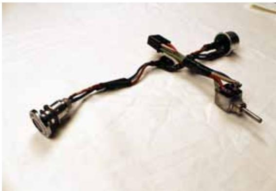
Modified hazard switch, indicator lamp, and flasher can assembly using terminals "C" and connector "B".
