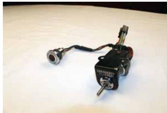
Modified hazard switch, indicator lamp, and flasher can assembly re-installed into the factory dash bracket.
