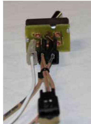
Figure "F" Dual fuel tank switch connection
