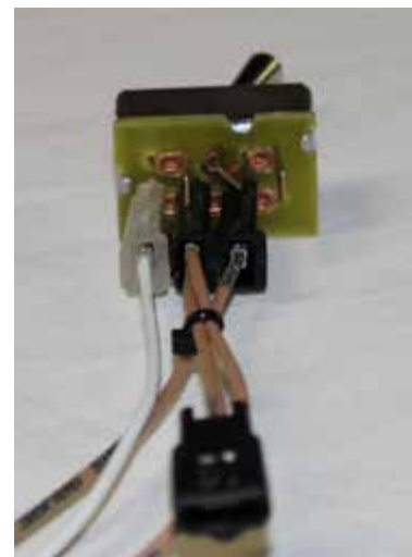
Figure "F" Dual fuel tank switch connection
