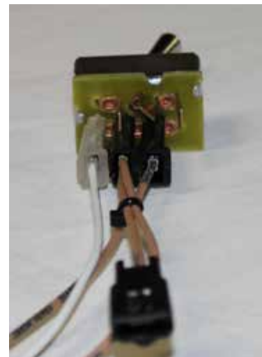
Figure "F" Dual fuel tank switch connection
