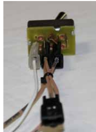
Figure "F" Dual fuel tank switch connection
