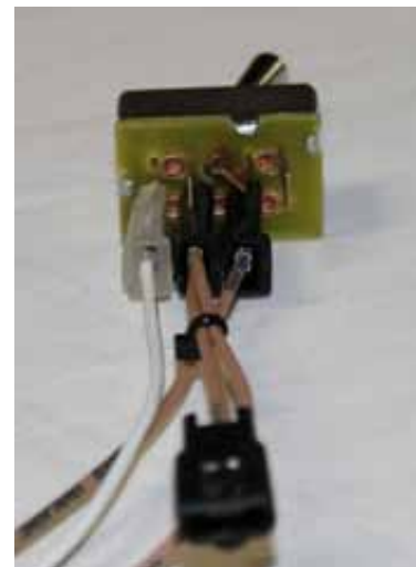
Figure "F" Dual fuel tank switch connection
