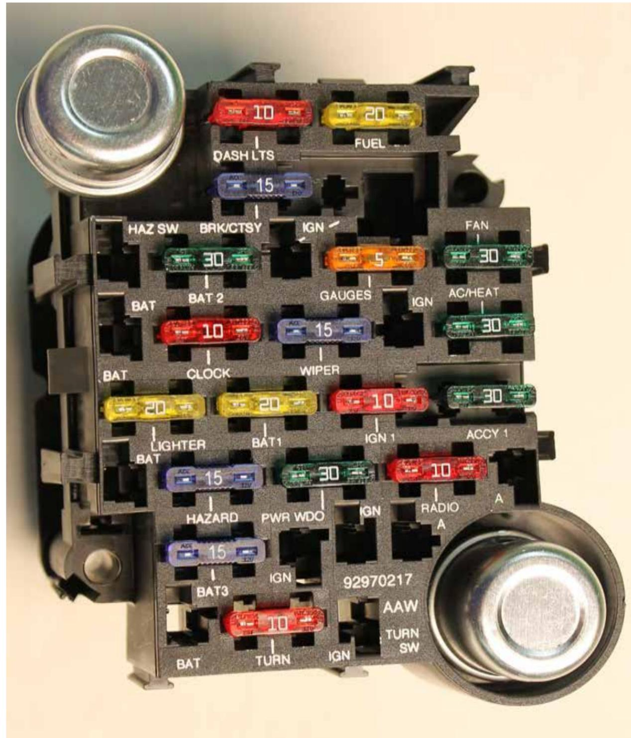
NOTE: Above, you will find a photograph of the completed fusebox assembly depicting the proper location for the installation of each fuse and the two flasher cans.
