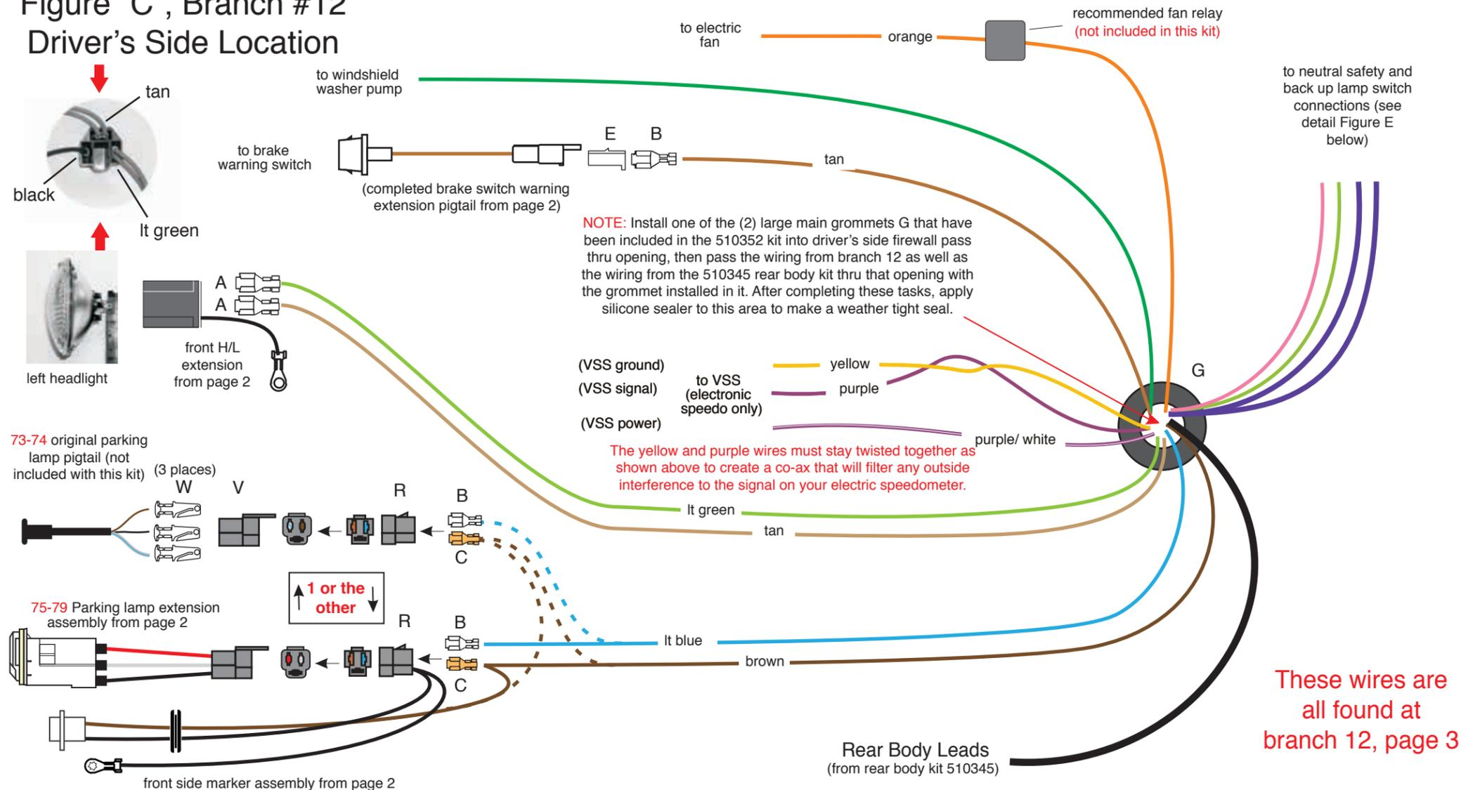
**NOTE:** Install one of the (2) large main grommets G that have been included in the 510352 kit into driver's side firewall pass thru opening, then pass the wiring from branch 12 as well as the wiring from the 510345 rear body kit thru that opening with the grommet installed in it. After completing these tasks, apply silicone sealer to this area to make a weather tight seal.
