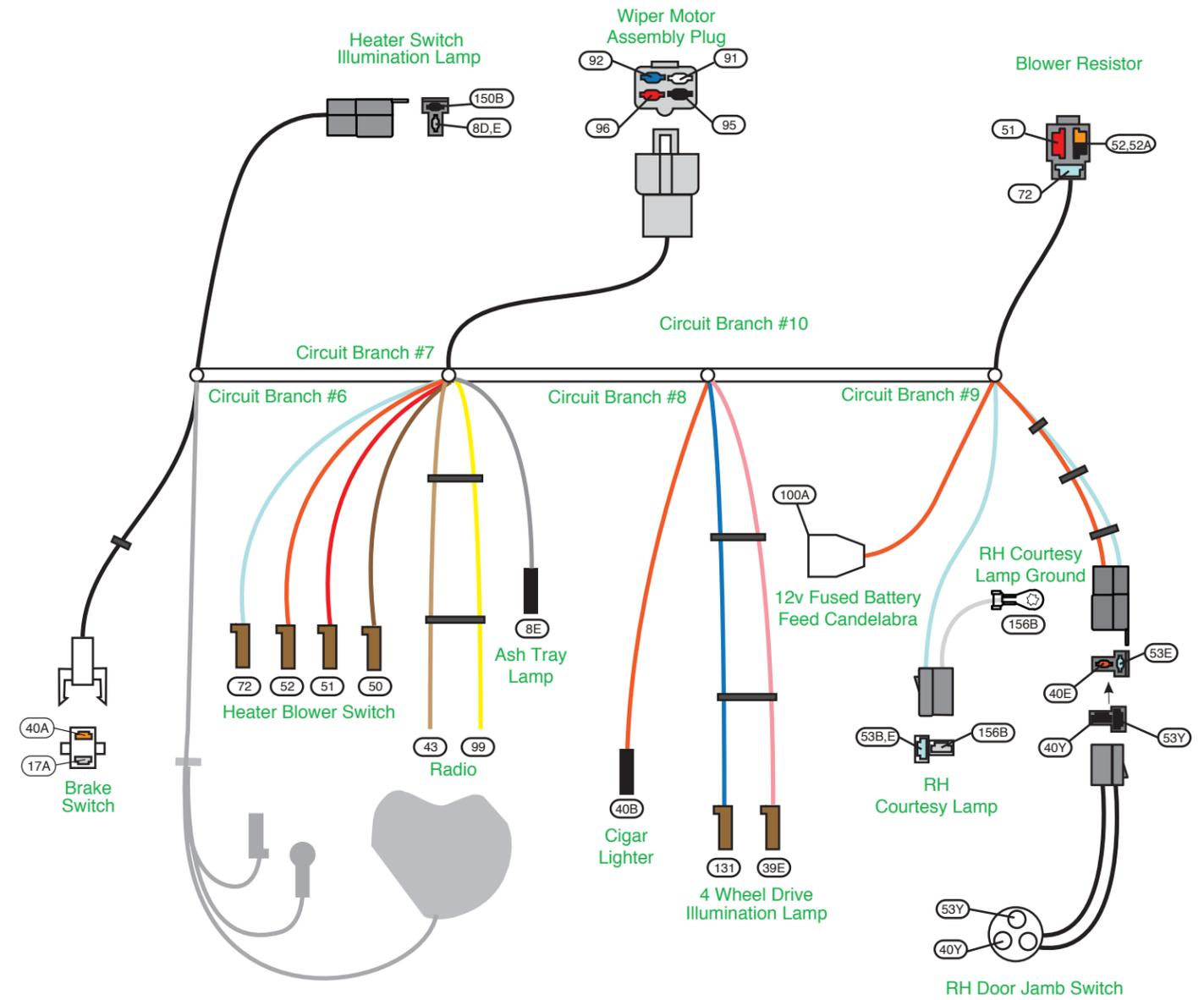
See page 7, Photo "A" for proper connector plug-in and orientation of Heater Blower Switch 50, 51, 52, and 72 wires (from above).
