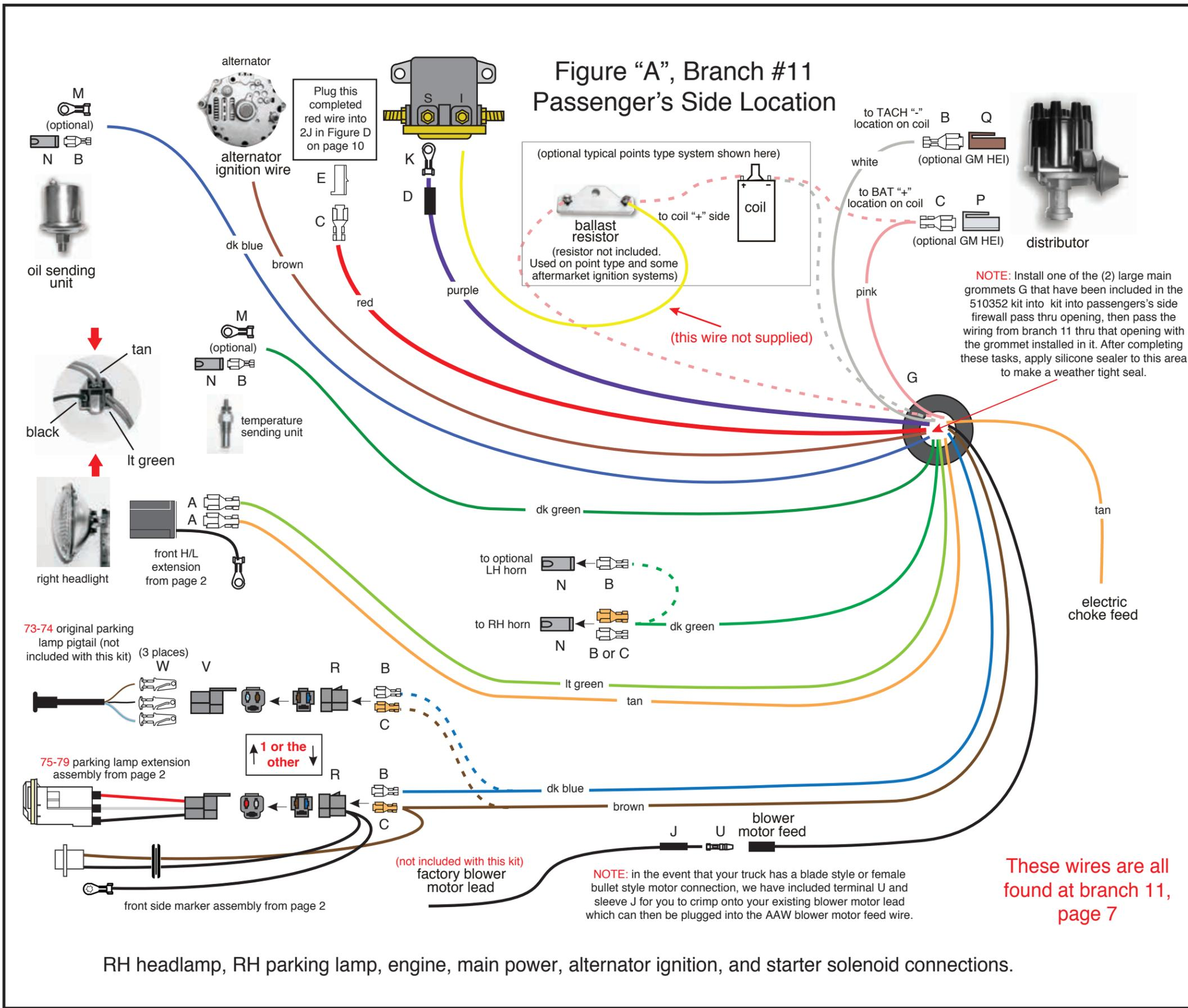
**NOTE:** Install one of the (2) large main grommets G that have been included in the 510352 kit into kit into passenger's side firewall pass thru opening, then pass the wiring from branch 11 thru that opening with the grommet installed in it. After completing these tasks, apply silicone sealer to this area to make a weather tight seal.
