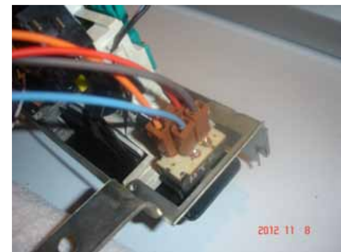
Photo "A" 1973 thru early 1978 (before serial number CA0001) heater blower switch connections (from page 6).
