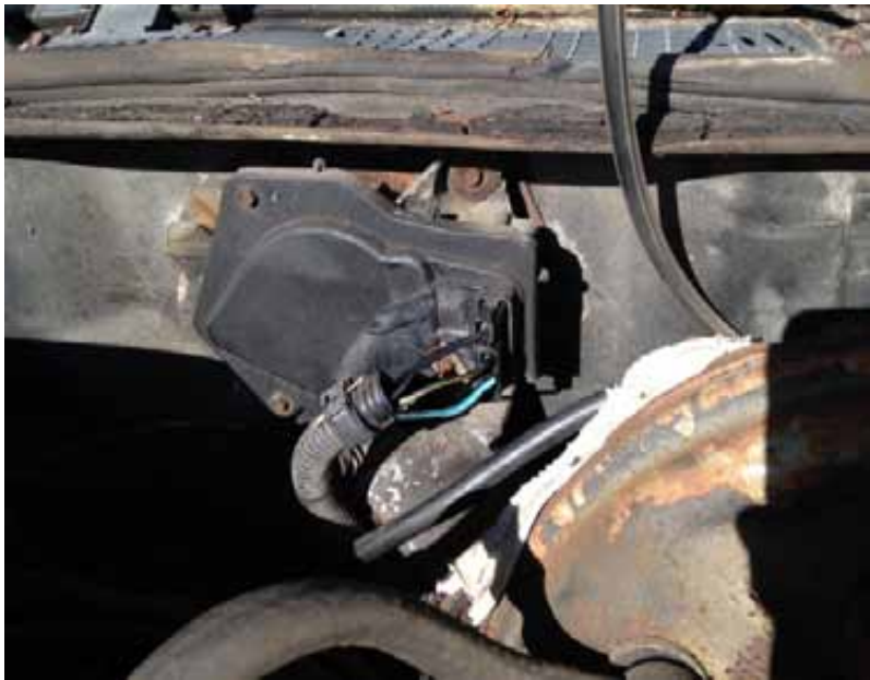
1975-1978 Camaro models with 2 speed wipers and washers. (Wiper motor connection shown. Washer pump is remote, is not shown, but can only be plugged in one way).
