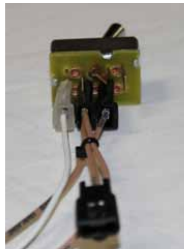
Figure "F" Dual fuel tank switch connection
