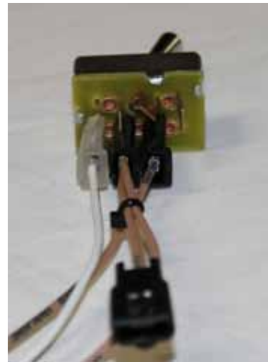
Figure "F" Dual fuel tank switch connection
