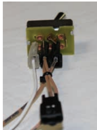
Figure "F" Dual fuel tank switch connection
