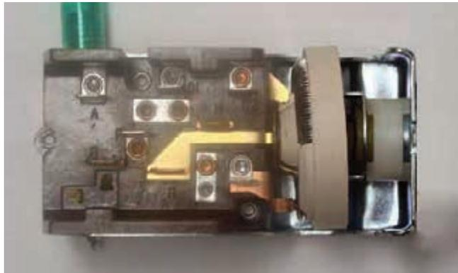
**NOTE 1:** If you are using this new AAW switch in a 1960 - 63 Falcon or a 1960-63 or 65 Comet, see page 1 of this instruction set. The switch installs with the connector area turned out to the LH driver's side as shown on page 1.
