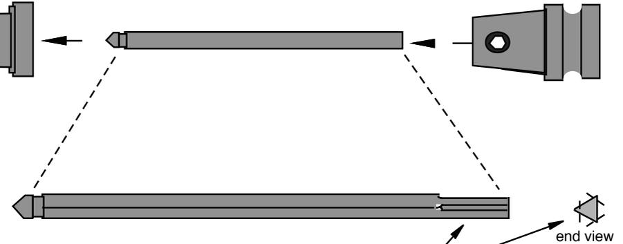
File shaft approximately as shown for proper fit on knob
