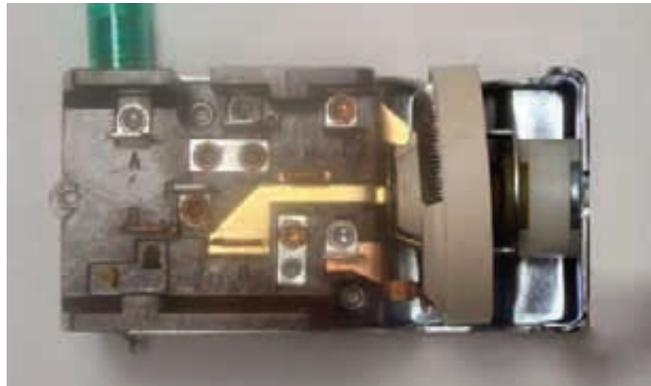
**NOTE 3:** Use this page of this instruction set if you are using this new AAW switch in a 1962 - 64 Fairlane or a 1962 - 63 Meteor. The switch installs into the dash with the connector area turned down toward the floor of the car as shown to the left.
