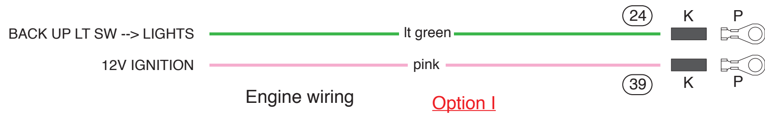
FIGURE "A" 1976-86 Back-up Light Switch Manual Transmission
