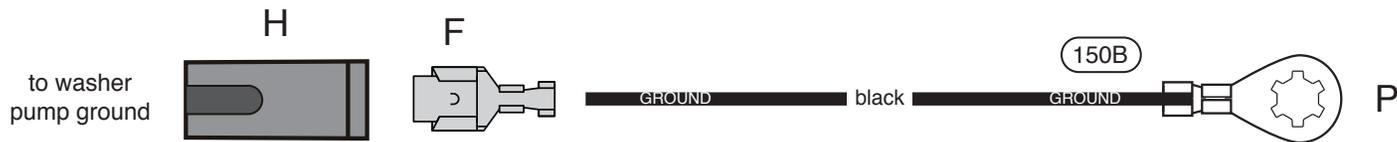
apply die-electric grease to the terminals, after all wires are installed
