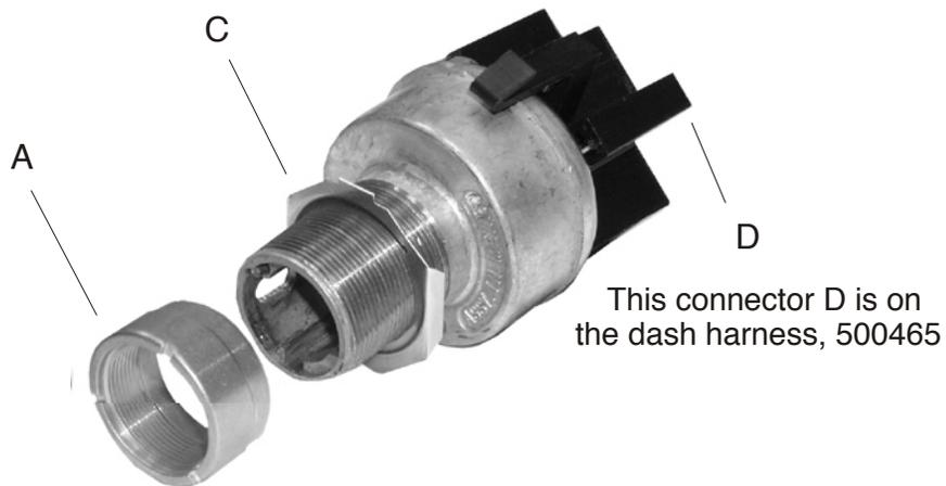
Completed ignition switch and dash mounting bracket assembly.
